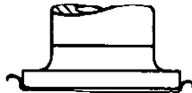
Fig. 4. No go segment of go and no go chuck fit gage partially seated in can end.
