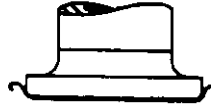
Fig. 5. Go segment of go and no go chuck fit gage fully seated in can end.
